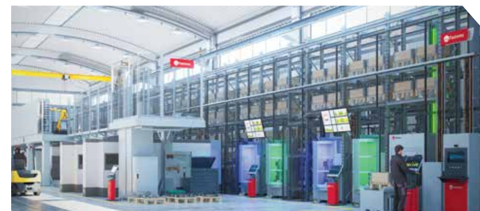
MLS GTS Full – The Fastems MLS Multi Level System features a Gantry tool storage, or GTS to automate tool processes.
